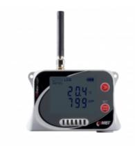
GSM datalogger is designed to record temperature, humidity, atmospheric pressure and CO2. In case of exceeded set limits, SMS and JSON messages can be sent via GPRS data connection. It is possible to set the regular sending of JSON messages to COMET Database, the sending interval is adjustable. Alarms are also indicated locally by LED, LCD and acoustically by built-in beeper.
